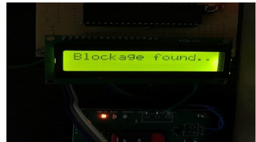
Figure 4 When the block occurs in the pipe it is detected and the display shows that blockage found.
