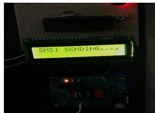
Figure 5 After detecting the block, the message is sent to the higher authority in municipality.
