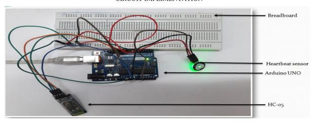
Above diagram represents the circuit connections of the components which includes Arduino Uno, Pulse sensor, Bluetooth module which in turn is connected to the computer.
