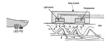
Photoplethysmography is a derivative of plethysmography technique, where in a simple optical setup can help detect volume changes in peripheral blood circulation. This technique is a non-invasive method since it makes measurements at the skin surface. The technology uses
