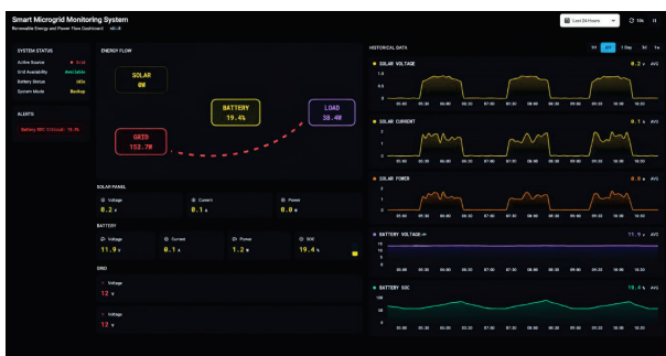
Fig. 10. Web-based dashboard showing microgrid (grid supply) operation during insufficient solar and battery conditions
