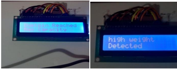
Fig8: output displaying on LCD board, dustbin reached maximum height and maximum weight.
