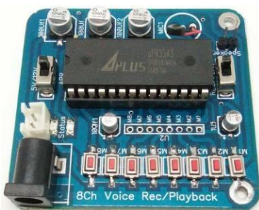
Fig-2: ARP33A3 Voice Recording and Playback Module
