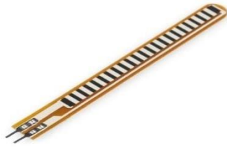
Fig-1: Flex Sensor
