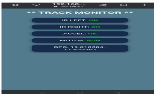
Fig. 3. Web dashboard showing real-time sensor status
