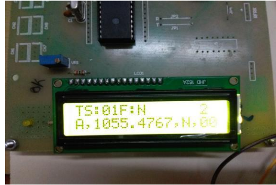
Figure: 5 LCD Module displaying the position using GPS
