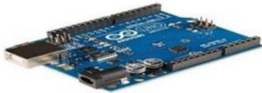
Fig.2 Prototype of Arduino Uno
