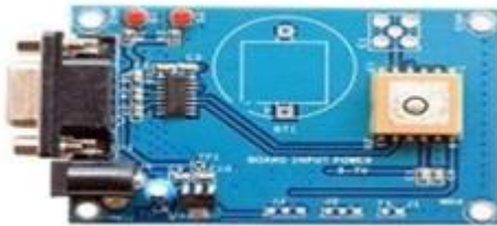
Fig.3 Prototype of GPS Module
