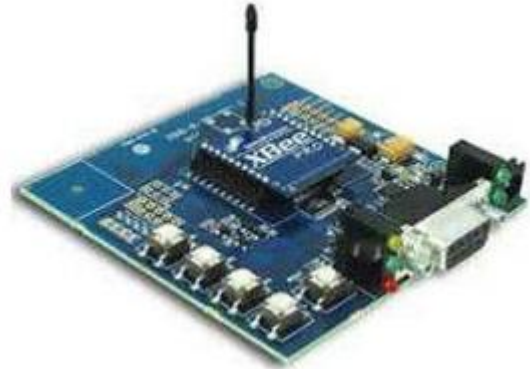
Fig.5 Prototype of Zigbee Module
