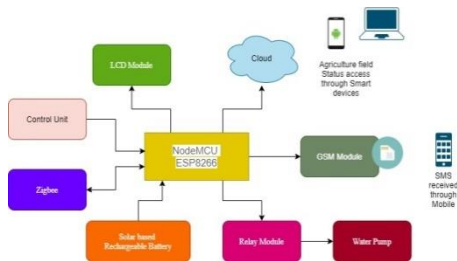
Figure 3 Block diagram of IoT based Master Node
