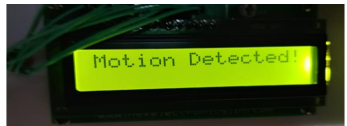
Figure 7.2 LCD displays the above message when the PIR motion sensor detects any movements
