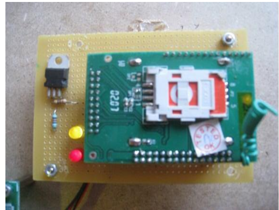
Figure 7 GSM Modem with SIM card for sending patient's data
