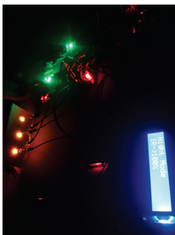
Fig. 9. Night Mode BRIGHT operation after IR motion detection.
