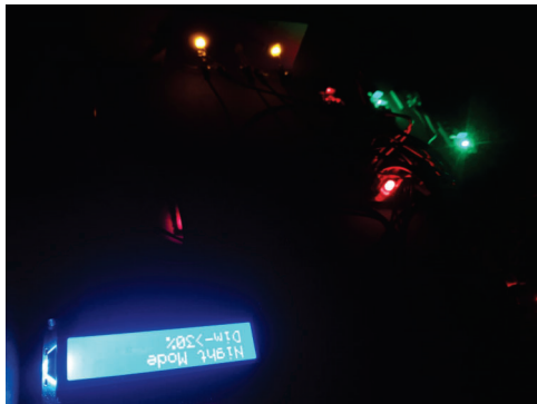
Fig. 7. Night Mode (DIM) operation with LEDs glowing at low intensity.
