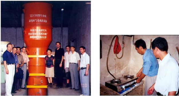
Figure 7. The Fluidized Bed Gasifier generating producer gas, developed in China
