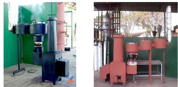
Figure 6. Gasifier Stove developed at AIT, IGS2 (left) and CGS3 (right)
