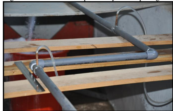
Fig 3.4 Experimental arrangement to find combined head loss
