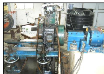
Fig. 4 Engine test set up
