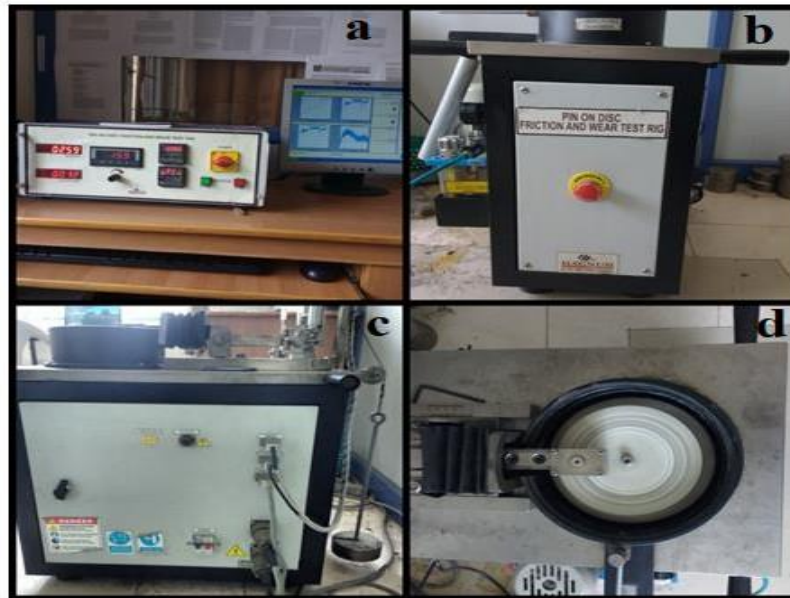
Figure 1 Friction and wear test rig (a) computer display (b) lubricant system (c) load setup (d) disc and pin holder
