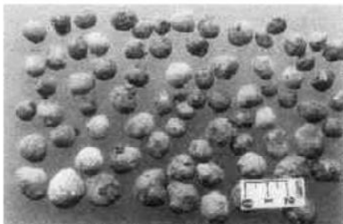
Figure 1 Photograph showing different size fractions and smooth surface of sintered pellets made from fly ash
