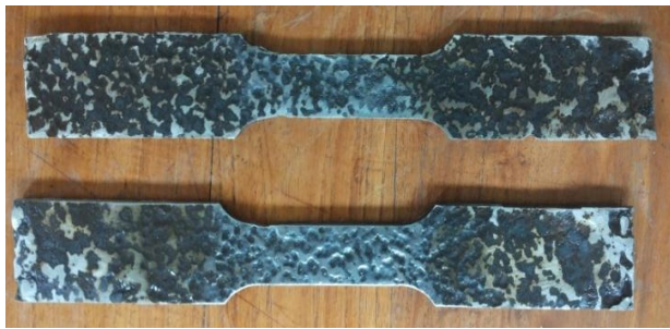
Fig. 2. Prepared test specimens according to standard shape
