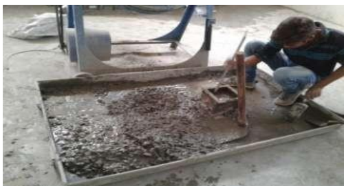
Figure– Casting of cube moulds with concrete
