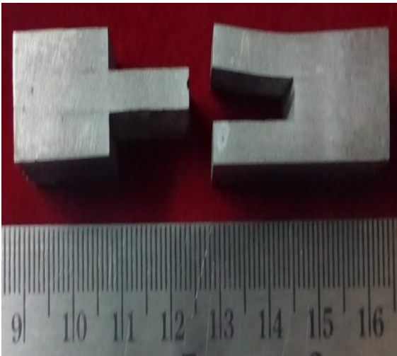
Fig. 2 Sheared base material
