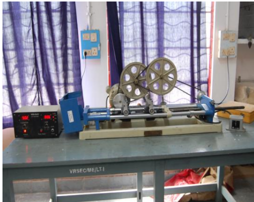
□ Φιγυρε 1: Shows the Tensometer for testing the Composite Specimens for both Tensile and Bending.
