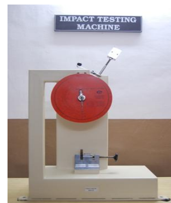
□ Φιγυρε 4: Shows the analog Izod/ Charpy impact tester for Testing the Composite Specimens (Impact)
