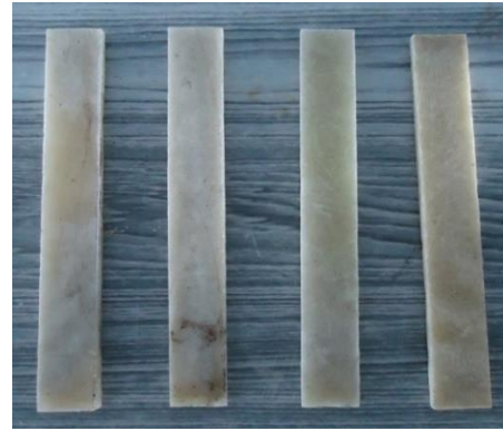
Fig. 2 Specimens of GFRP laminate with dimensions of 250 \text{ mm} \times 30 \text{ mm} \times 8 \text{ mm}
