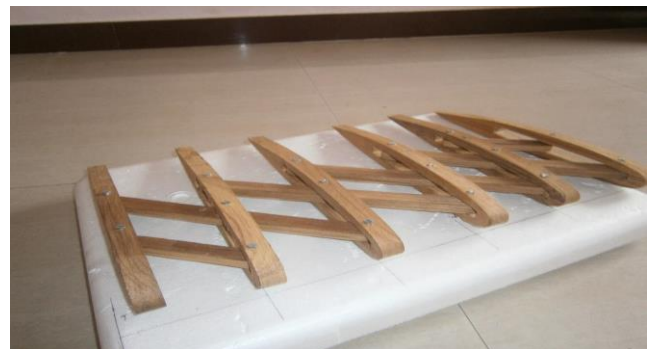
Fig 7.2 Prototype of the internal structure of morphing wing
