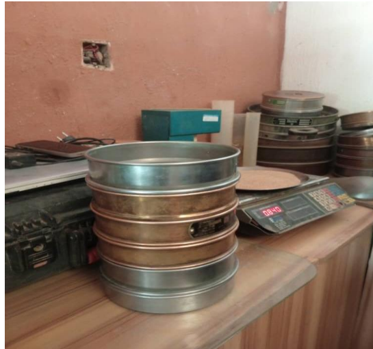
Plate 4. Sand sample undergoing sieve analysis.
