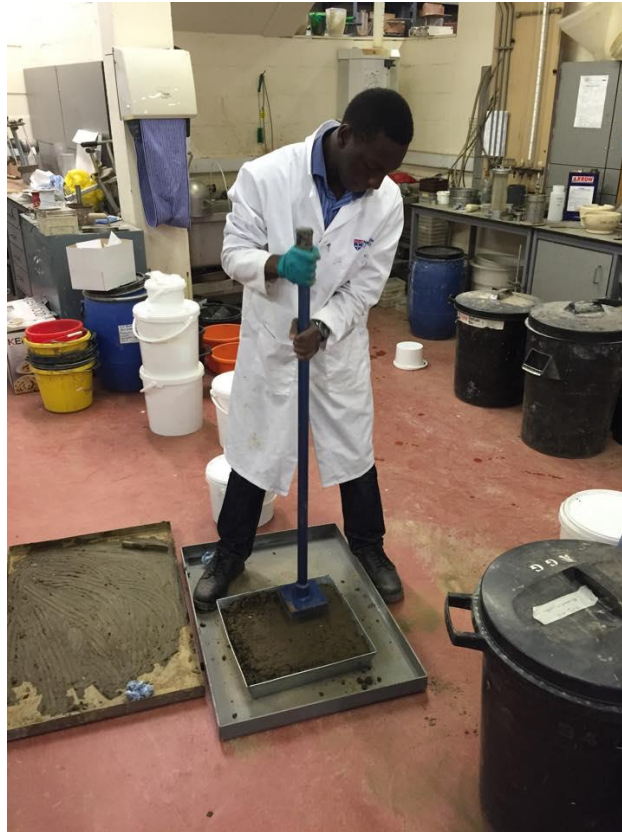
Figure 3.2: Sample preparation by tamping with a square base hammer
