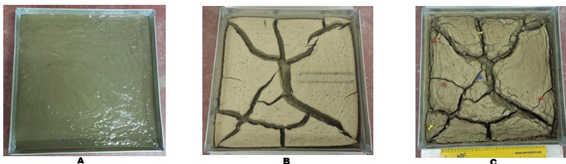
Figure 4.3: Validation of cracks in a slurry sample (A): Slurry at the start of the experiment (B) After oven drying at 110°C (C) Second drying cycle at 110°C
