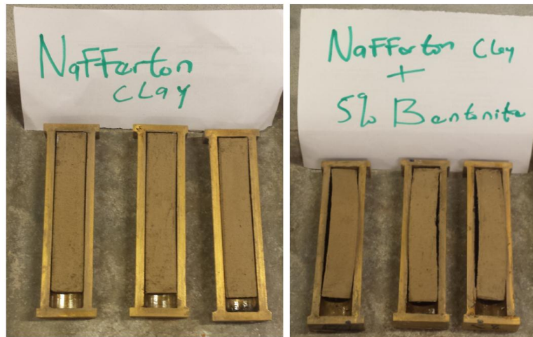
Figure 4.2: Linear shrinkage test (note the higher plasticity sample has curled)
