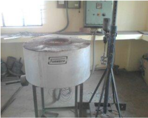
Fig.1. Stir casting setup
