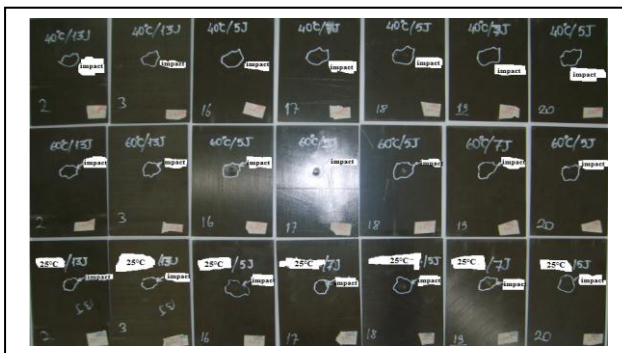
Figure 6. Samples subjected to low energy impact test at +25°C, +40°C and +60°C respectively
