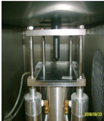
Figure 5. Settlement of sample to the fixture
