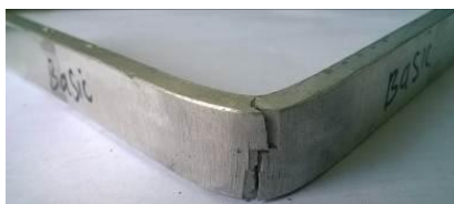
Fig. 16. Bend tested base alloys AA7075-T6.
