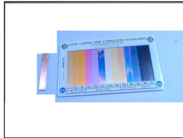
Figure 8. Copper strip corrosion test for transformer oil with 100 ppm Irgamet 39 compared with ASTM colour code.
