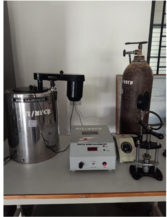
Bomb Calorimeter -A thick – walled steel container used to determine the energy contained in a substance by measuring the heat generated during its combustion.
