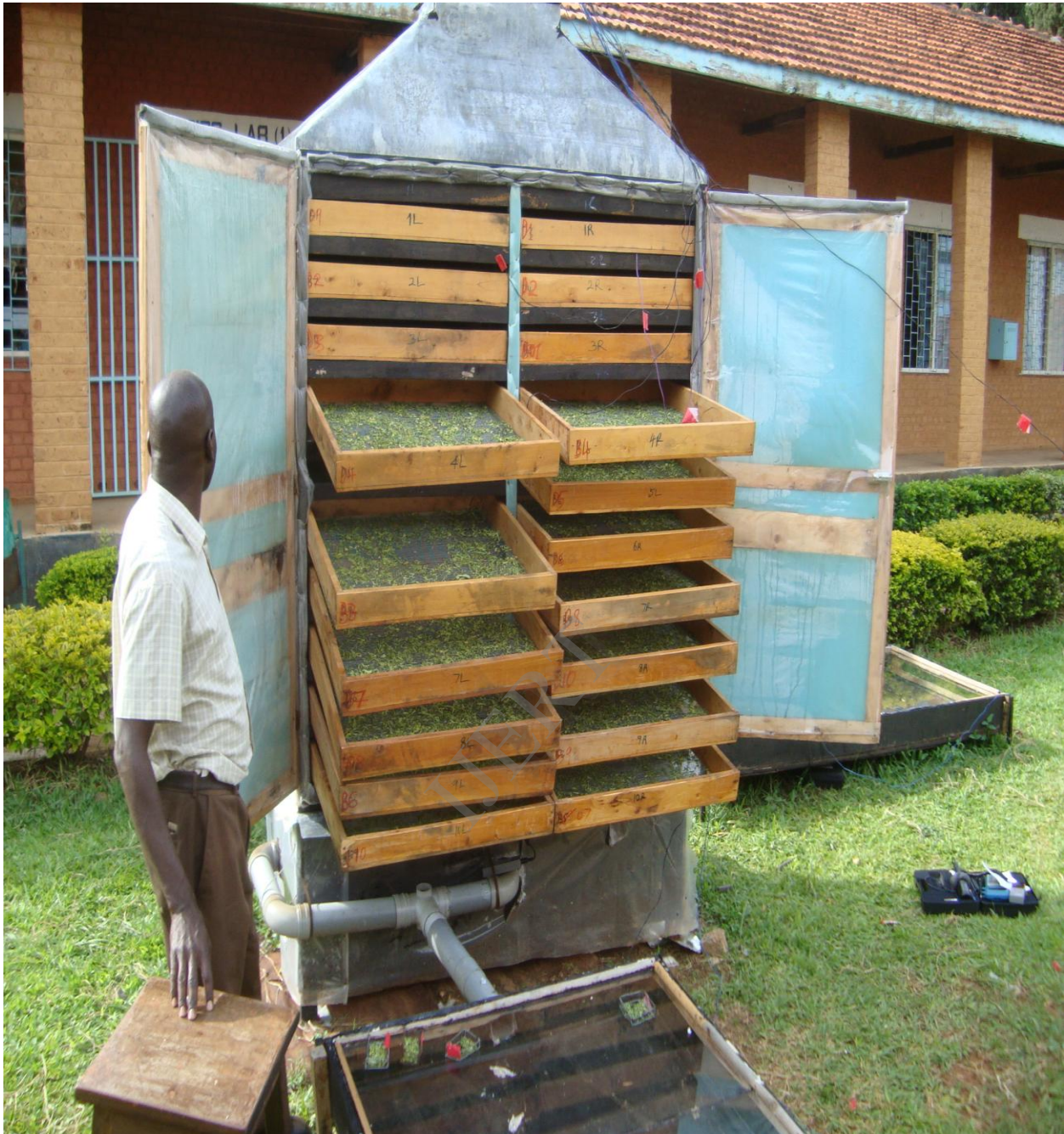
Figure 1: Pictorial view of the indirect cabinet solar dryer designed at the Department of Physics and Materials Science, Maseno University, Kenya.
