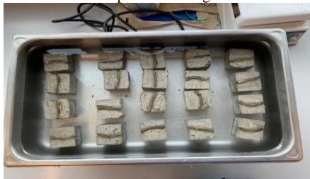
Fig. 4. Concrete samples being boiled to dissolve PVA wedges
