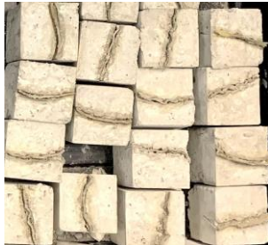
Fig. 3. Photo of concrete samples after being taken out of the mold
