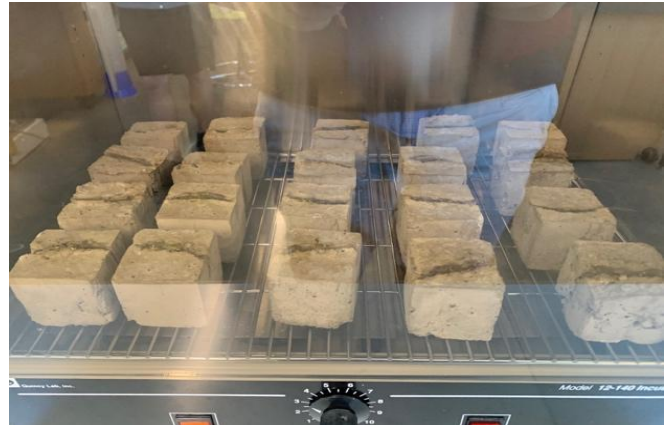
Fig. 5. Concrete samples being incubated in natural daylight conditions
