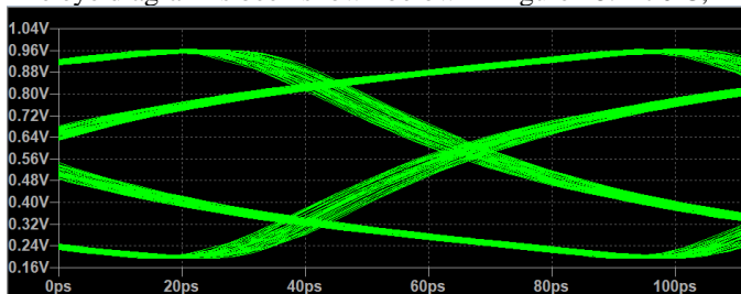
Fig. 18 Eye diagram of the circuit at 0 °C
