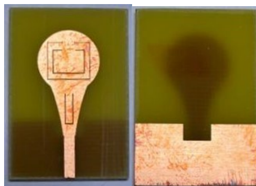
Fig. 6: Fabricated Triple Band Notched UWB Antenna Source: IUM Fabrication Laboratory
