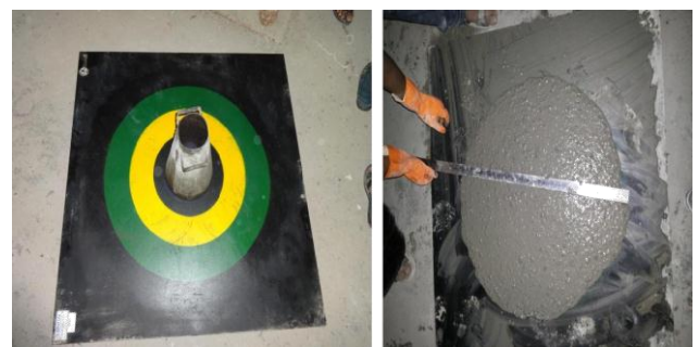
Figure 1 Slump Flow Test
