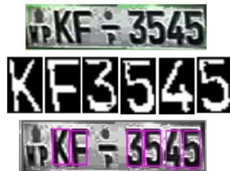
Fig 1: Recognized Number Plate and segmented characters
