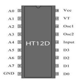
HT12D is a decoder integrated circuit that belongs to 212 series of decoders. This series of decoders are mainly used for remote control system applications, like burglar alarm, car door controller, security system etc. It is mainly provided to interface RF and infrared circuits. They are paired with 212 series of encoders. The chosen pair of encoder/decoder should have same number of addresses and data format.
