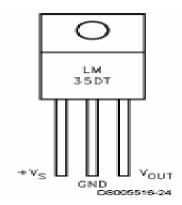
Calibrated directly in ° Celsius (Centigrade). Linear + 10.0 mV/°C scale factor. 0.5°C accuracy guaranteable (at +25°C). Rated for full -55° to +150°C range. Suitable for remote applications.Low cost due to wafer-level trimming. Operates from 4 to 30 volts.Less than 60 µA current drain.Low self-heating, 0.08°C in still air.Nonlinearity only ±1/4°C typical.Low impedance output, 0.1 W for 1 mA
