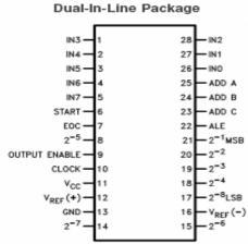
The ADC0808, ADC0809 data acquisition component is a monolithic CMOS device with an 8-bit analog-to-digital converter, 8-channel multiplexer and microprocessor compatible control logic. The 8-bit A/D converter uses successive approximation as the conversion technique.
