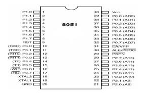
The microcontroller is the heart of this system. The microcontroller used here is 8051 family (AT89C51). It is a 40 pin, 8bit microcontroller. RAM 128 bytes, ROM 4 KB. It has 4 ports, and one serial communication.
