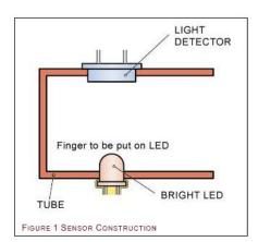
This heart beat sensor is designed to give digital output of heat beat when a finger is placed inside it. When the heart detector is working, the top-most LED flashes in unison with each heart beat. This digital output can be connected to microcontroller directly to measure the Beats Per Minute (BPM) rate. It works on the principle of light modulation by blood flow through finger at each pulse. Heat beat
