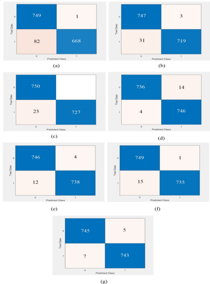
Figure 6: shows the confusion matrices for (a) SqueezeNet, (b) AlexNet, (c) GoogLeNet, (d) ResNet-50, (e) DarkNet-19, (f) DenseNet-201, and (g) ShuffleNet.
