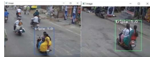
Fig. 6. Real-time results of helmet and triple riding detection
