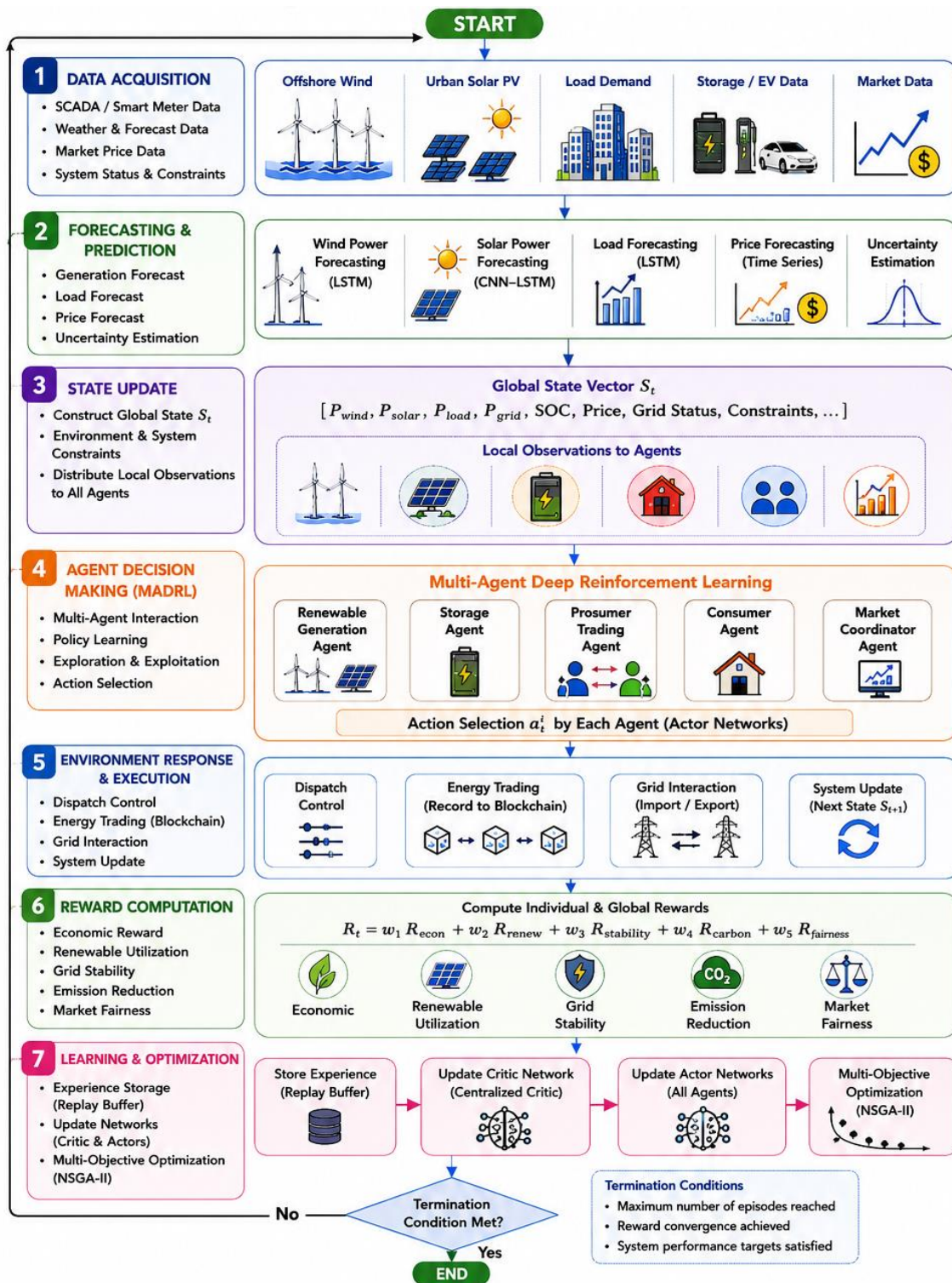
Figure 2. Flow Chart of the Proposed Intelligent Smart City Energy Ecosystem Based on Blockchain-Enabled Peer-to-Peer Renewable Energy Management, Multi-Agent Deep Reinforcement Learning, and Multi-Objective Optimization.
