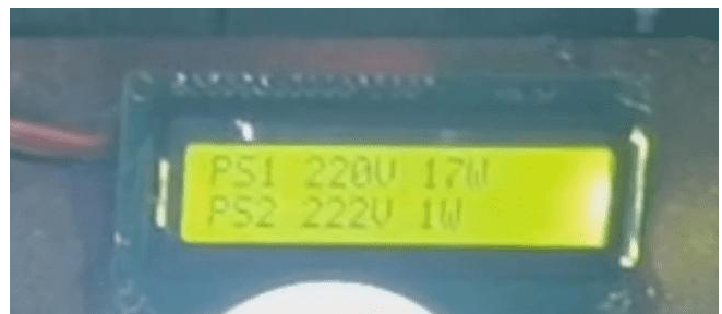
Fig. 8. LCD display output for local monitoring.
