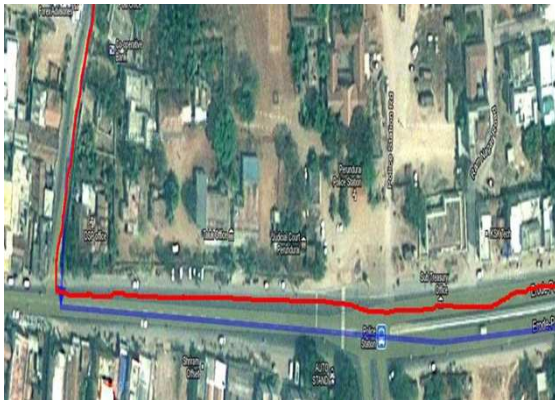
Figure:10 Path(along with divider) tracked by INS-GPS system
