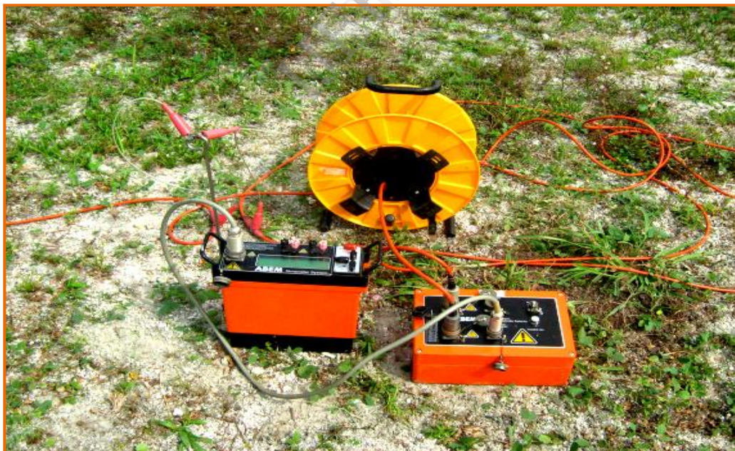
Figure 9: viewing the instrument type SAS1000 applied in geophysical survey
