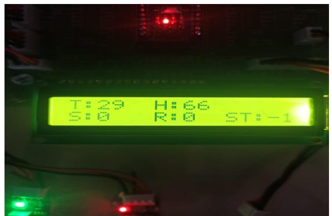
Fig. 4. Displaying Temperature, Humidity, Soil moisture, Rainfall and Soil temperature
