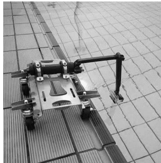
Figure I-5 The cart position on the side of the swimming pool, as used in the experiment.
