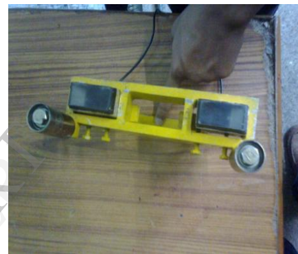
Fig: 700 probes in side probing frame
