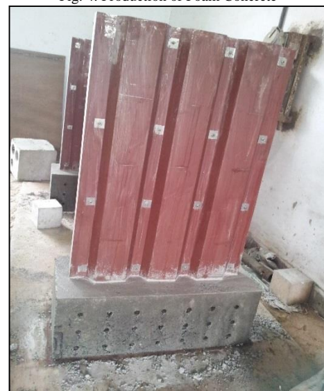
Fig. 5. Casted panel with base concrete
