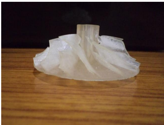
Fig 13 Impeller prototype produced using SLA process
