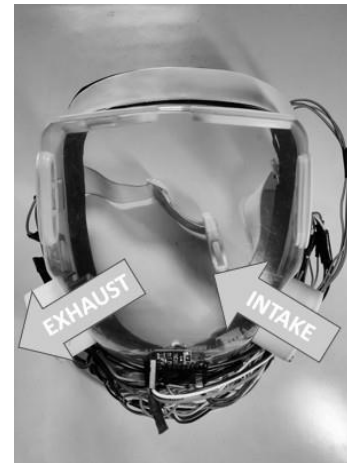
Fig. 3. Basic air ventilation process
