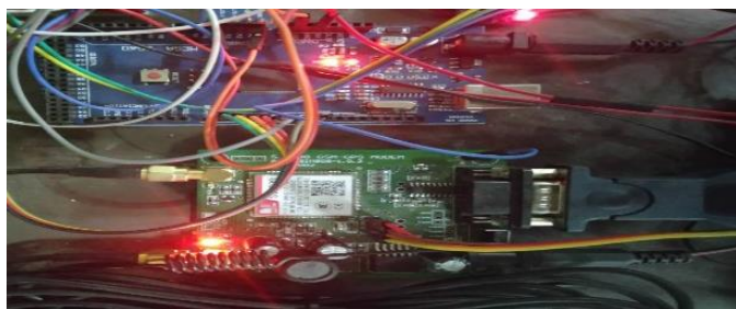
Fig -6: Interfacing GPS-GSM Modem with Arduino
